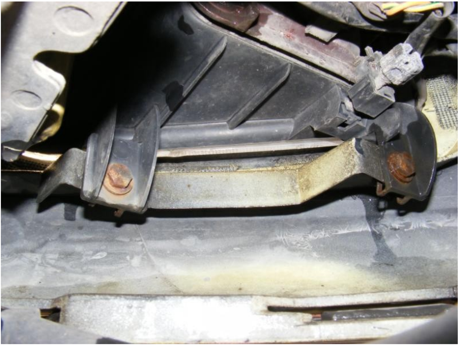
Bulb holder, connector & the silvery thing sticking off the bottom of the lamp housing is the level adjuster:
