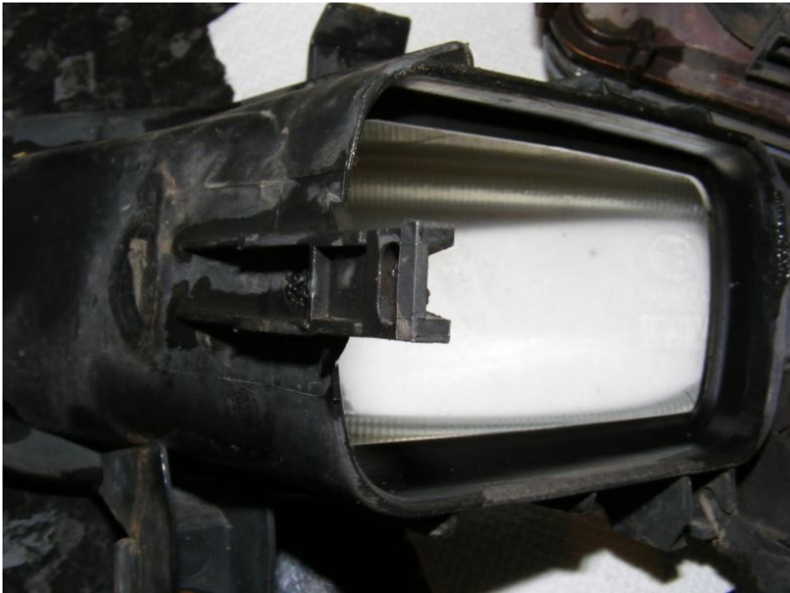
The plastic lug (1 on each side) on the inside part of the lamp once removed:
